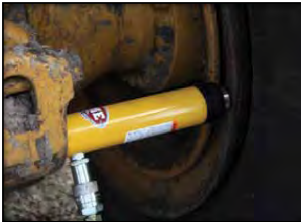
Hydraulic rams are used to break the back beads on earthmover wheels
