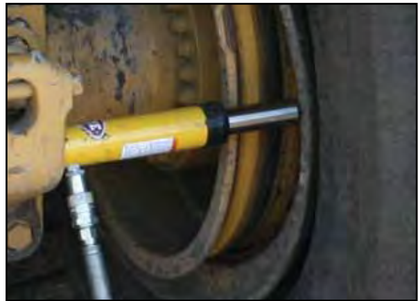
Hydraulic rams are used to break the back beads on earthmover wheels
